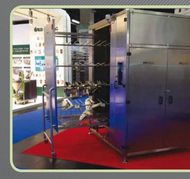
A typical wash cycle includes a hot pre-wash at between 50°C and 55°C followed by a recirculated detergent wash at the same temperature. To ensure efficient cleaning of the weigh pans and ancillaries, the washing chamber is equipped with IWM's proven and effective motorised TravelJet system, which incorporates corrosion-proof plastic bayonet type water jets or, optionally, stainless steel jets.
