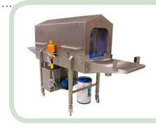
They feature solenoid-controlled proportional injector pumps to ensure efficient and accurate dosing of sanitising fluid and incorporate bayonet fitting spray tips that can be removed easily for cleaning or replacement. The body of the machines is fabricated throughout from T304/316 stainless steel, and their robust streamlined design allows easy access to all areas for routine cleaning – including a newly designed removable top canopy cover.
