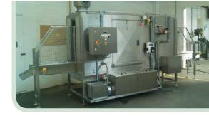
The overall design of the machine has also been upgraded to maintain its robustness, ensuring that it will have a long reliable life even in tough operating conditions, while eliminating flat surfaces, joins and creases in its construction, making it easier to clean and improving its hygienic characteristics. These improved characteristics make the new machine particularly well suited for applications in the food and pharmaceutical sectors.
