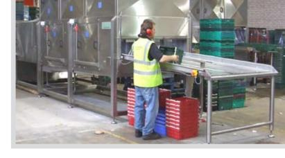
blow-off sections are fitted, plus one heated section to allow the trays to be delivered dry and ready for immediate use. IWM further customised the T1500 by re-designing the in-feed system so that it would accept trays from a raised platform rather than from ground level.
