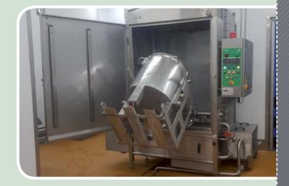
a cold rinse, using a solenoid-controlled supply of fresh water from the mains. EC20-30 bin washers are constructed from stainless steel throughout to ensure that they are robust and have a long working life. They feature a streamlined design that is not only hygienic, but also allows easy access to all areas for cleaning and maintenance. Based on proven technology, they are competitively priced and are backed by IWM's renowned maintenance and support services.
