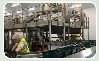
For the new manufacturing facility, IWM supplied a continuous washer for 200 litre Eurobins, a twin-track high-care tray washer for cleaning the wide variety of trays used to transport raw ingredients around the facility, and five cabinet utensil washers for depositor parts, salad bowls and similar items.
