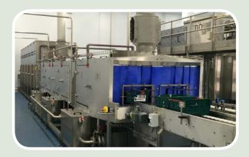
Operators place nested stacks of dirty trays on to the stack infeed of the Autarky destacker which then elevates the stacks before removing individual trays from the top of the stack. The separated trays are then inverted to allow loose debris to fall from the trays before being turned upright and conveyed to the washer.
